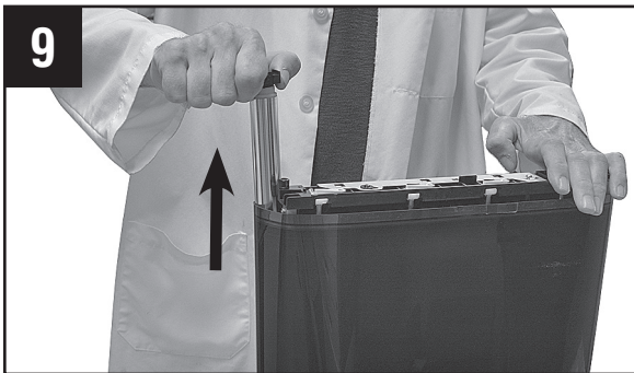
9 Remove the tension roller by sliding it up and out.
